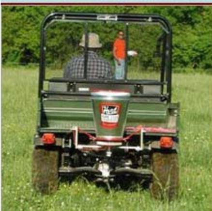
Applying fire ant bait using a herd seeder mounted on an ATV.
