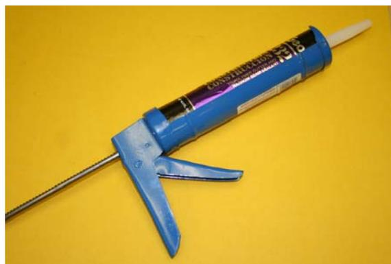
Sealants containing siliconized latex or ethylene copolymers are usually a good choice for sealing small gaps. Photo credit: UT E&PP, K. Vail.
